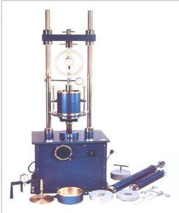
**Gambar 3** Alat Uji CBR Laboratorium
